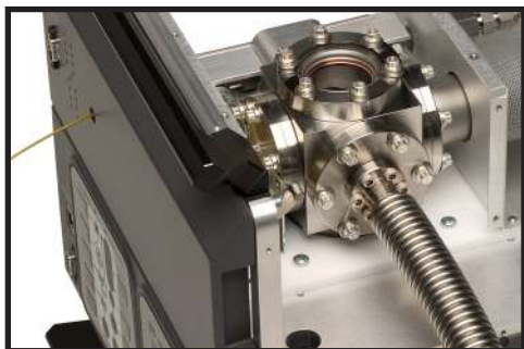
Direct connection for UHV applications
