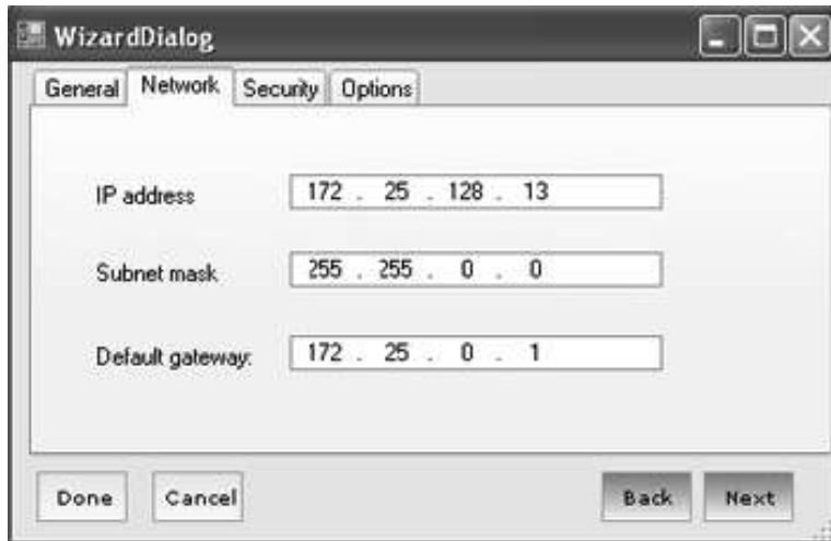
Fig. 2-5. Screenshot of the 'Network' tab in the 'Wizard' dialog box.
