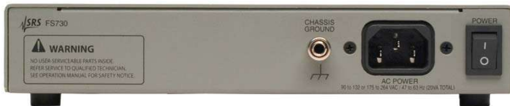
Figure 2. Rear panel of FS730 Distribution amplifier.
