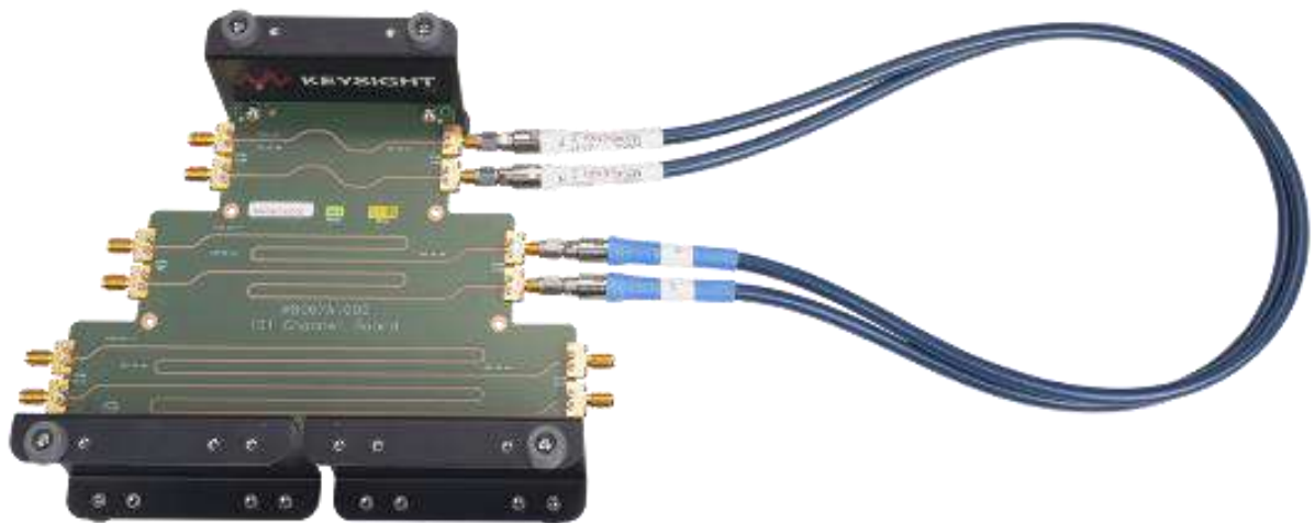
Figure 4. To achieve higher insertion loss, you can cascade two ISI channels by connecting them with a cable.
