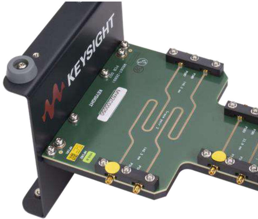
Figure 3. The 1.0 mm connectors are soldered, and the connectors have a mechanical hold.
