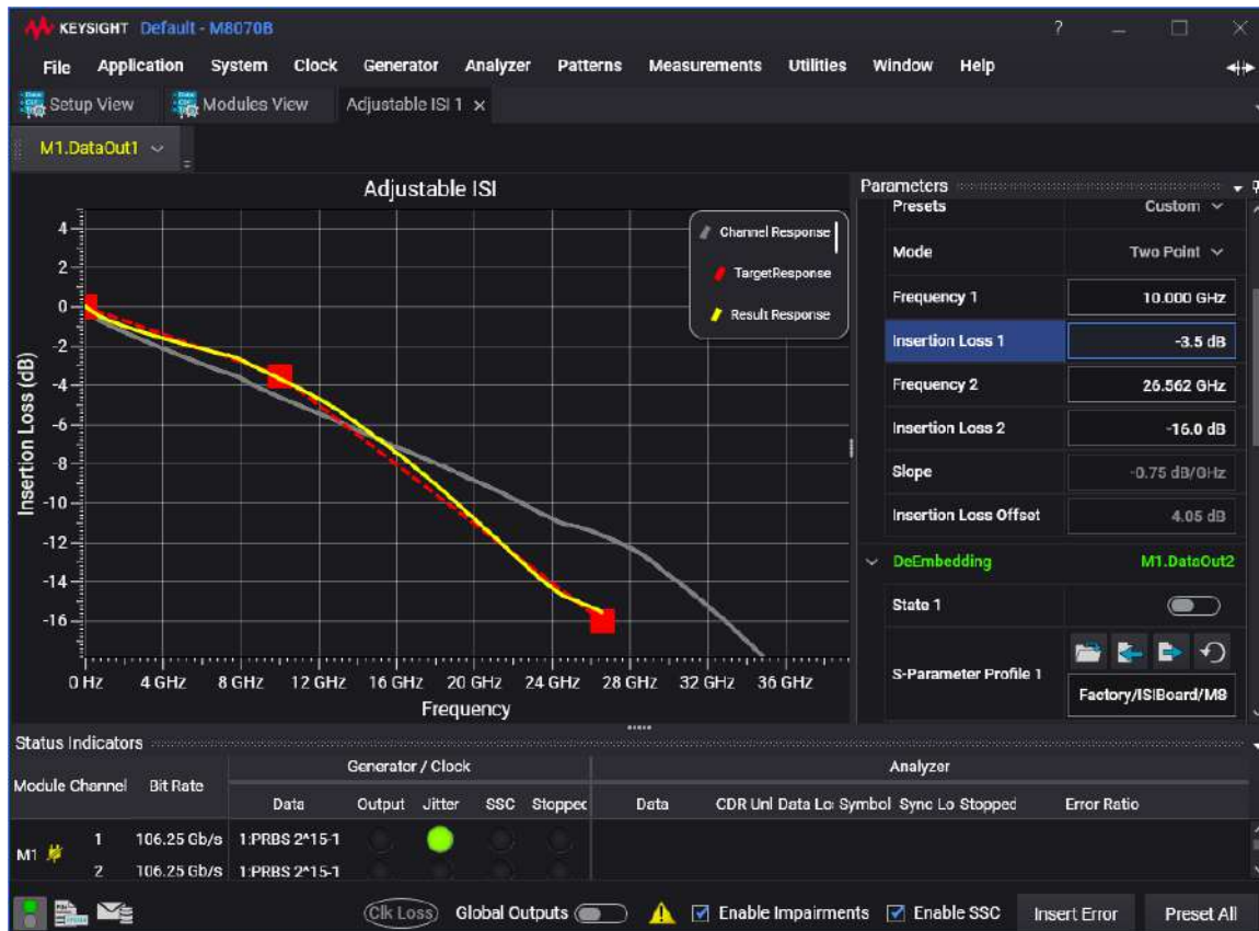
Figure 12. The adjustable ISI software package M8070ISI allows to emulate ISI internally with the M8042A pattern generator module. The example shows as channel response (gray) the insertion loss of an external ISI channel. You can add or remove insertion loss (red for target response) at 2 frequency points.
