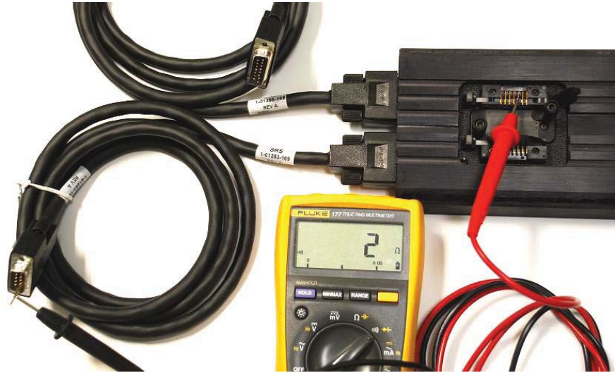
Figure 2.4: Verifying correct wiring prior to use.
