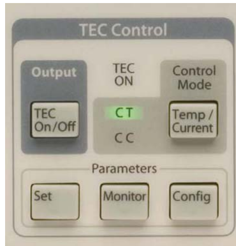
Figure 2.5: The TEC Control block.
