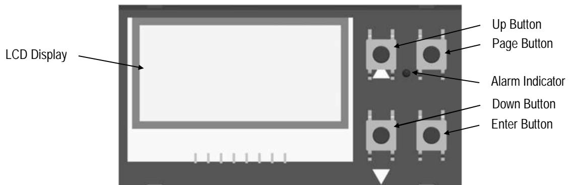
Figure 33: Control Panel for the Comm Box (DIN)
