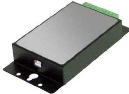
Figure 52: USB/RS485 Adapter (XXXUSB485)
